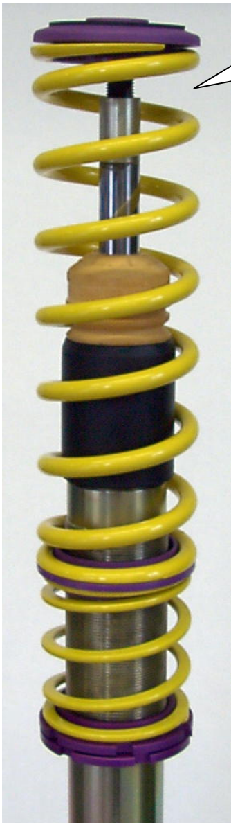
Angeliefertes KW Federbein Supplied KW coilover strut
