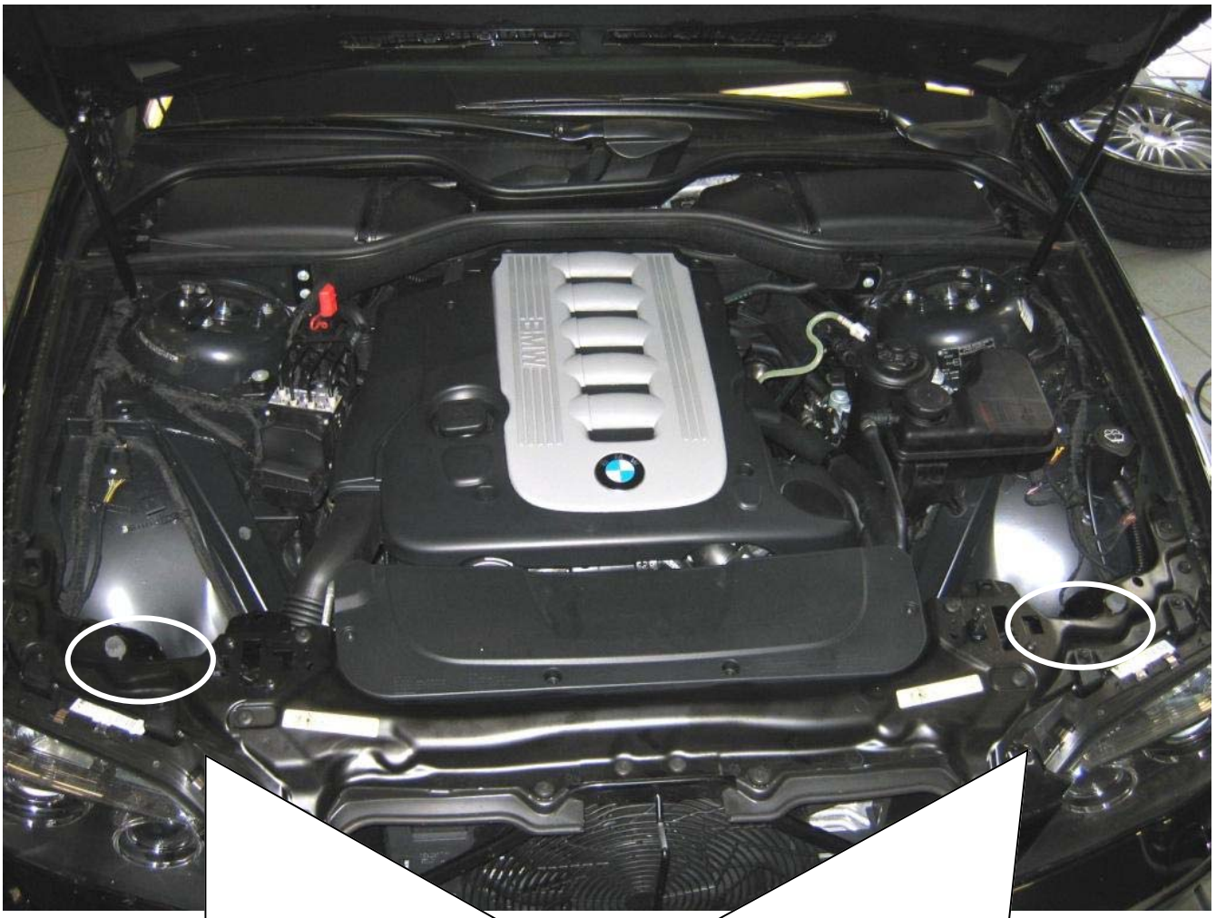
Montageort VA Elektroniksatz / Assembly site front axle electronic kit
