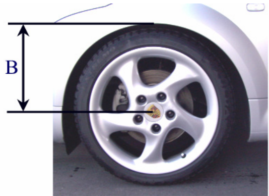
Measurement B Wheel hub center wheel arch
