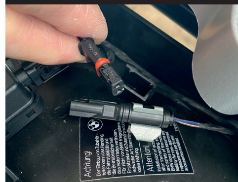
Four pin indicator connector rear location
