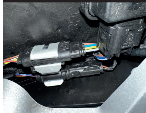
Four pin indicator connector rear location
