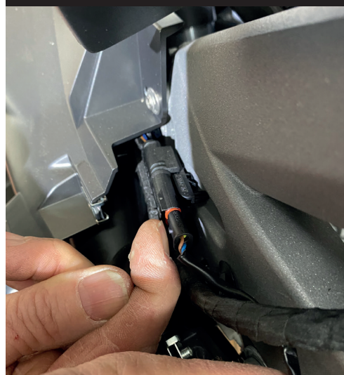
Two pin indicator connector front location
