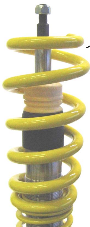
Angeliefertes Federbein. Supplied coilover strut
