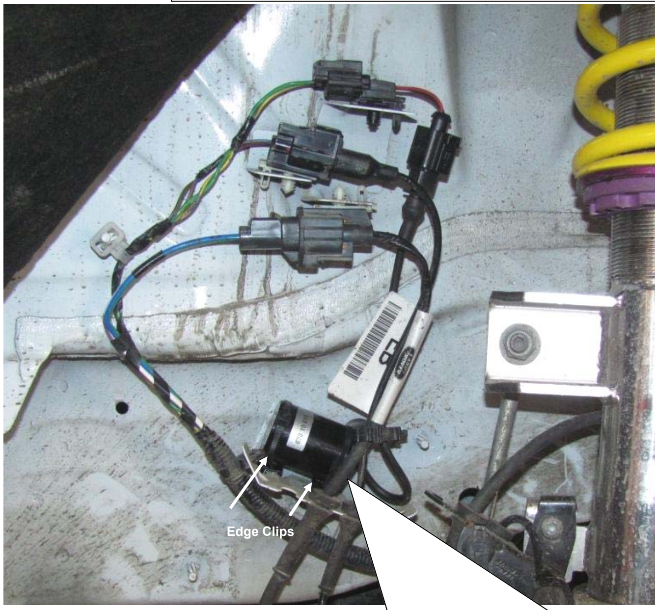
Montageort VA Elektronik Satz / Assembly area front axle electronic kit
