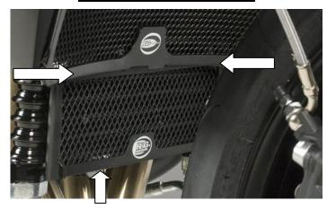
In This Kit There Should Be 1x Oil Cooler Guard (OCG0009) 2x 100mm Lengths of Foam
