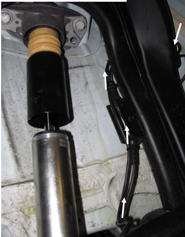
Montageposition 3 / Assembly position 3
