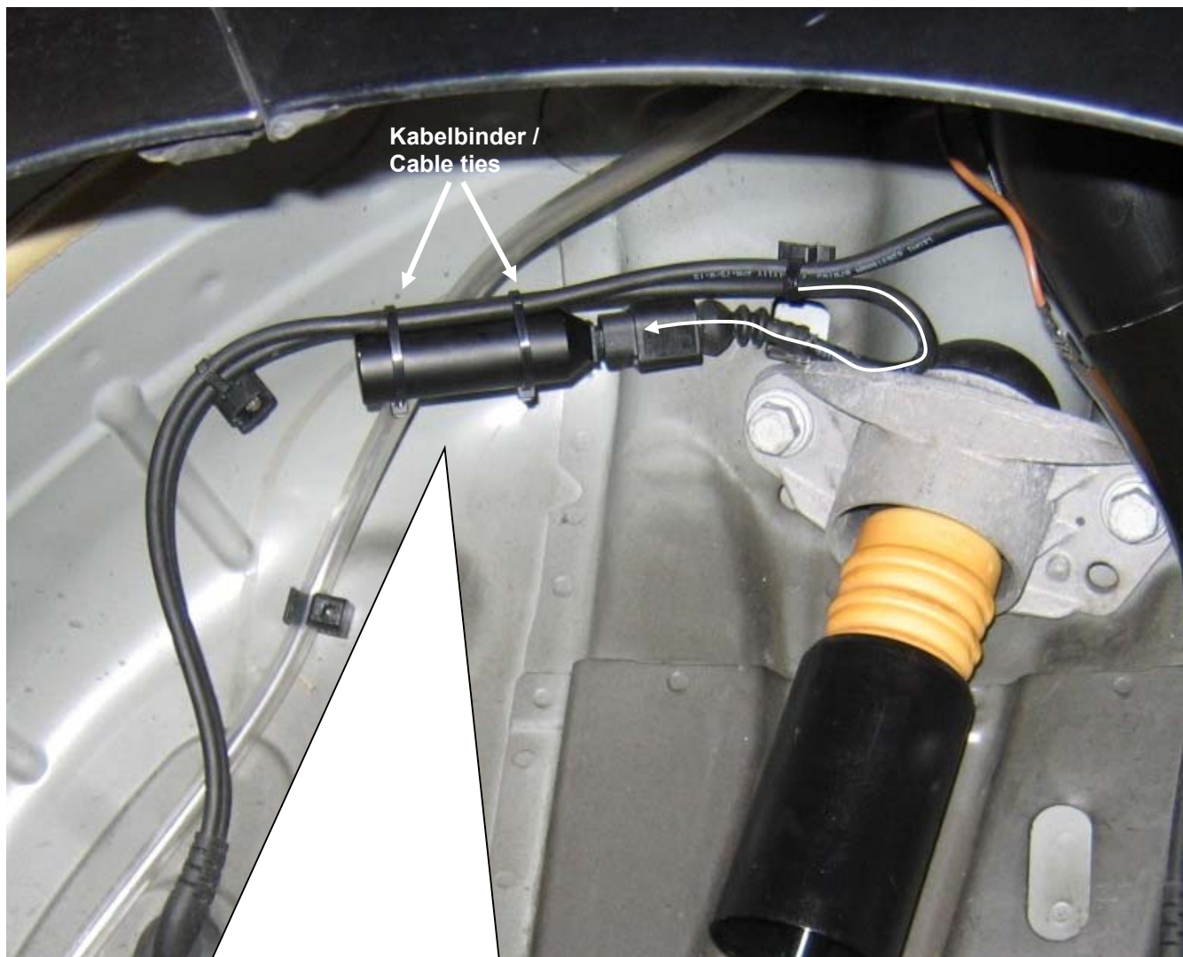
Montageort HA Elektronik Satz / Assembly area rear axle electronic kit
