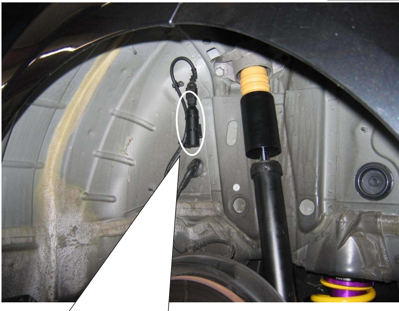
Montageort HA Elektronik Satz / Assembly area rear axle electronic kit
