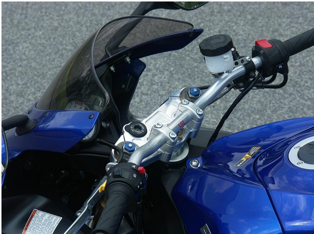
**i** To avoid scratches and dents when re-routing hoses and cables remove the fuel tank first. Remove fairing bracket and mirrors if necessary. The battery ground should be disconnected before working on electric wiring and switches!
