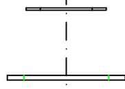
Rondelle / Washer  $\varnothing$ 28mm
