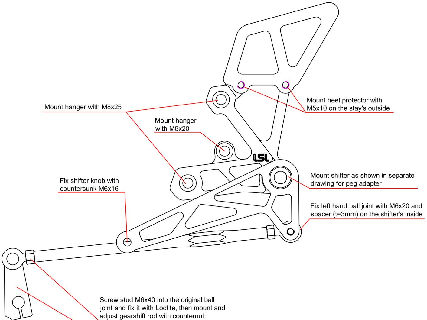
**Advice: Turn gear-box lever upside down for reversed shifting!**
