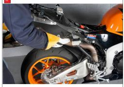
Q) Remove x2 bolts that hold the the O.E silencer.
