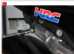
I) Remove the plastic cover, push fit connection.
